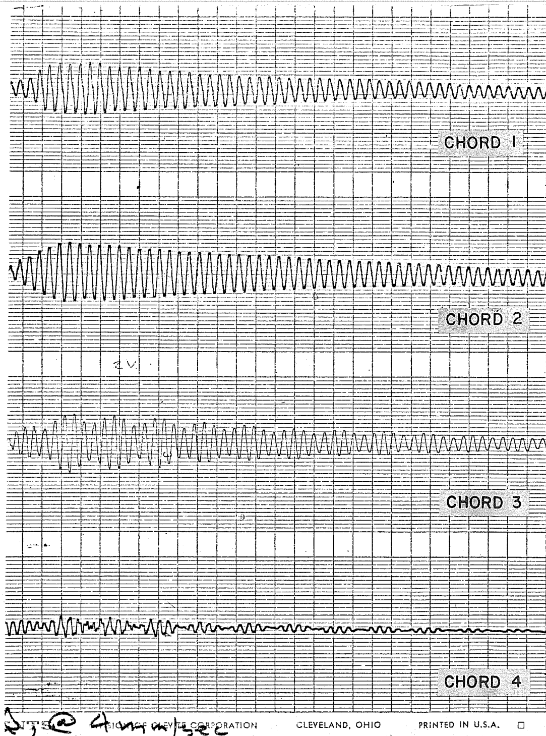
Fig. 3.6 Strain traces from a vertical forced vibration test of single cantilever sign
